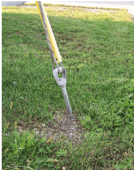
5/8 Inch (1.6 cm) Diameter; 16,000 Lb Force (71,171 N) Ultimate Tensile Strength; Rod with assembled eyenut
