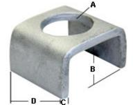
MacLean galvanized steel bond clamps provide a sturdy and efficient provision to connect ground wire to threaded bolts. The clamps are designed to nest over the square nut of the bolt. The grounding connection is accomplished by inserting the ground wire between the nut and the bonding clamp and adding an additional nut to secure the clamp and ground connection. The clamps accommodate the most common range of ground wire diameters.
