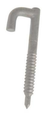
Drive Hook 7/16" diameter x 4 3/4" long. Hooks used to attach wedge type service drops and deadend clamps to crossarms, poles or buildings. Hook is furnished with 7 /16" fetter drive threads and a pilot point for easy starting.
